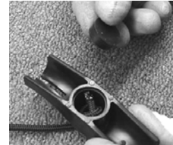
Remove the plug in the handle. Untie the knot in the rope. Slip the rope out of the handle.
